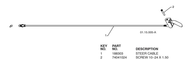
**NOTE:** All component dimensions given in U.S. inches. 1 inch = 25.4 mm **IMPORTANT:** Use only Original Equipment Manufacturer (O.E.M.) replacement parts. Failure to do so could be hazardous, damage your snow thrower and void your warranty.
